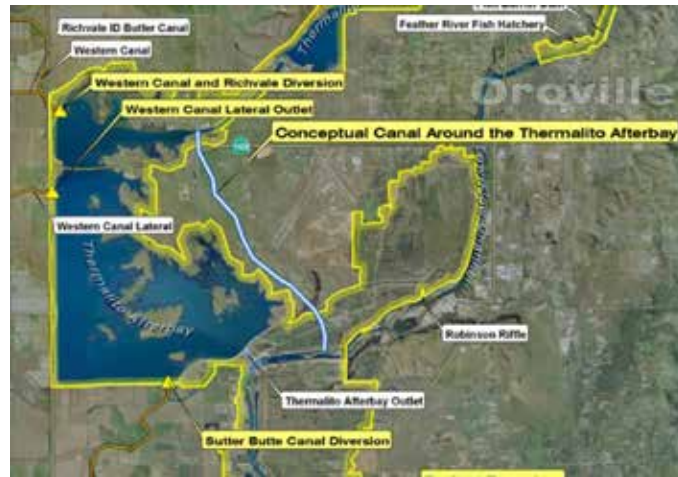
This slide is from a recent DWR presentation showing the conceptual canal that would convey cold water back to the Feather River, opening 15 miles to spawning
